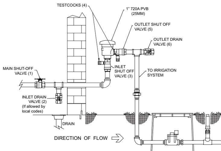
The discharge should cease by the time the shut-off valve is in the full open position.
