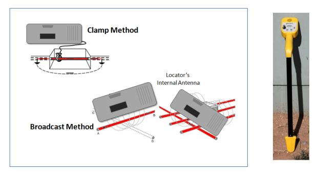
Once a tracing current has been induced in the cable, the cable path can be followed using the receiver wand. The pickup coils in the tip of the wand sense the magnetic field around the cable producing an audible tone and a meter indication on the wand control panel.
