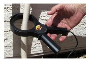
Note: For best performance orient the clamp with the wired handle closest to the tracked cable. See photo.
