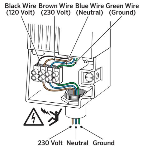
4. Strip about ½" (13 mm) of insulation from the end of each AC power wire.
