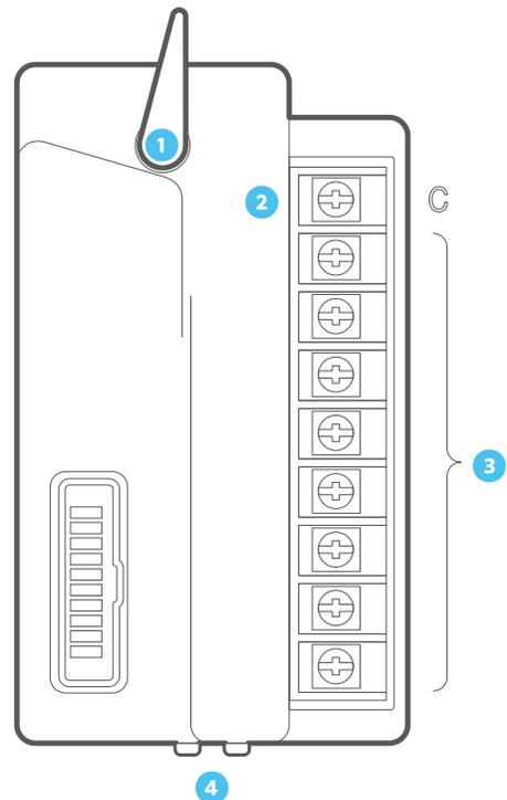
The ICM2200 expansion module increases overall station count to 38 (plastic) and 54 (metal). This module can be installed exactly like the ICM400 and ICM800 station modules; however, it covers two station output slots.
