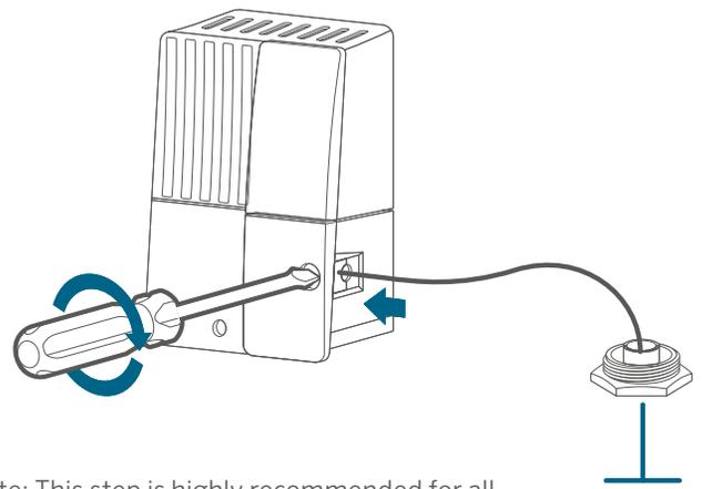
Note: This step is highly recommended for all installations, and is required to properly ground metal and SS configurations.
