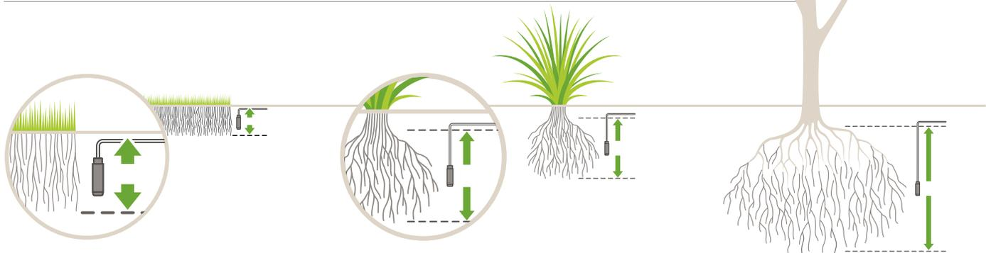
In turf applications, the probe should be placed in the root zone, approximately 6 inches deep (adjust for actual turf conditions).
