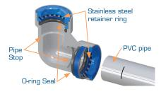
When PVC pipe is inserted to the Pipe Stop, the o-ring seals around the pipe and the stainless steel ring "locks" the pipe in place.
