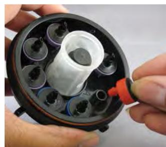
**NOTE:** Always install the emitters with the pointed or threaded end UP.
