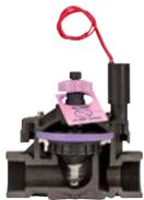
The ICV-R glass-filled nylon reclaimed water valve is optimized for non-potable water applications. The diaphragm is made from chlorine-resistant EPDM rubber, which significantly lengthens the valve's field life. Filter Sentry® comes standard with the ICV-R, keeping the diaphragm filter screen free of debris often found in reclaimed water.
