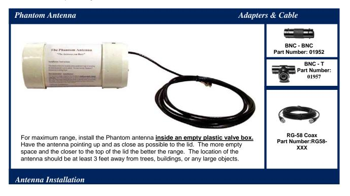
Successful wireless communication range is achievable in most locations as long as these installation practices are observed. TRC Irrigation Remotes can supply connectors and RG58 Coaxial Cable in lengths from 3, 10, 25, 50 and 100 feet (specify when ordering). Your range will be maximized by following these guidelines:
