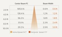
Beam angle is calculated using LM-79 method for SSL Luminaires:
