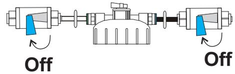
**Step 2** - Open the drain valve allowing for depressurizing and drain until empty. Remove the fill cap to allow for faster draining
