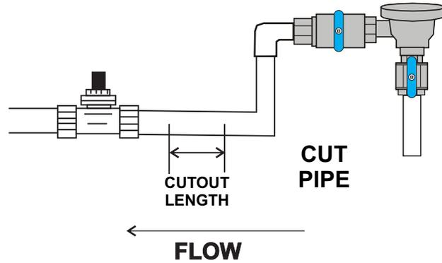
**Step 4 - Glue the coupling into the line.**
