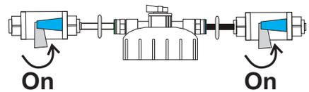
Allow the tank to pressurize and view all connections for leaks
