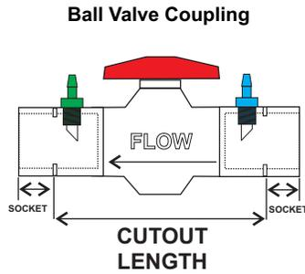
**GLUE IN COUPLING WITH FLOW ARROW POINTING IN THE DIRECTION OF THE WATER FLOW**
