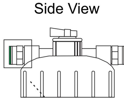
The EZ-FLO system uses push connect fittings to connect the clear and black 1/4" tubing to the cap.
