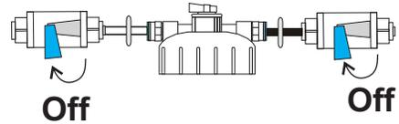
Turn water on at back flow preventer opening valve slowly to minimize hydraulic shock / water hammer.
