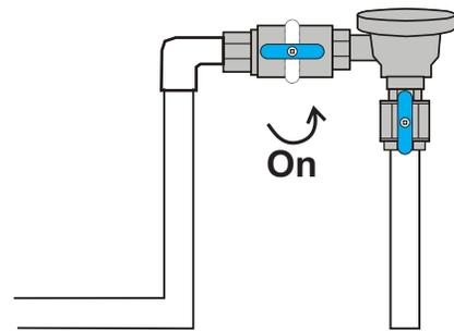
Turn on both shut off valves at the proportioning cap
