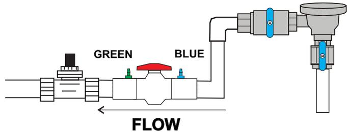
**Step 5 - Attach tubing to the coupling.**
