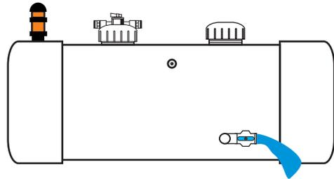
**Step 3** - Remove Fill Cap & Close Drain Valve
