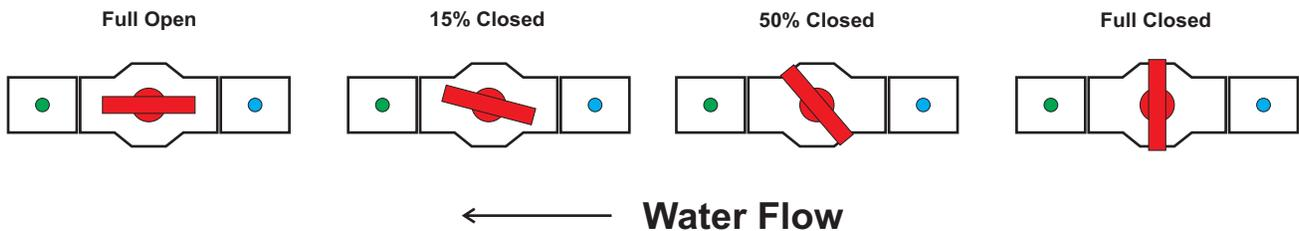
Once color is visible, you no longer have to adjust the CBV connection. You may leave it in position permanently. **Full closed is not common and may indicate improper installation or filling of the system.**
