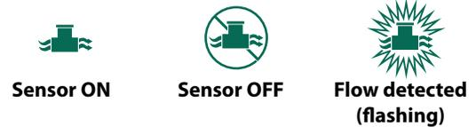
**NOTE:** When switching from **Sensor OFF** to **Sensor ON**, the controller will begin to LEARN FLOW. It will run each station for short period to set the expected station flow.
