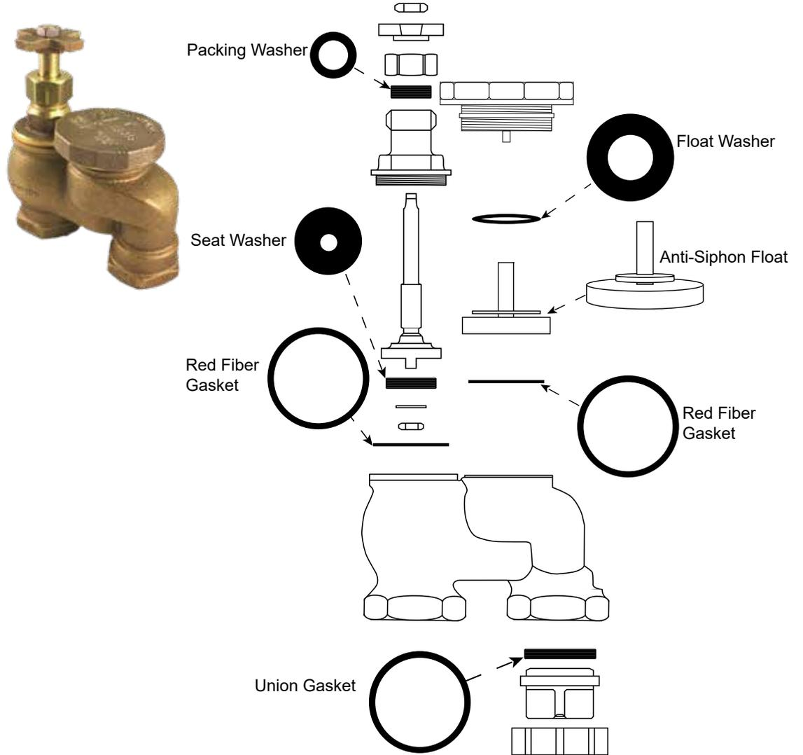
\*In order to rebuild, both the brass anti-siphon cap and the manual stem must be removed.
